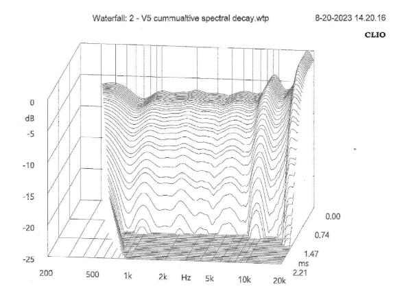
CSD: 1/3 Octave Spectra No. 60 Time Step 0.037ms Rise Time 0.576ms File: V5 cummualtive spectral decay.wtp
