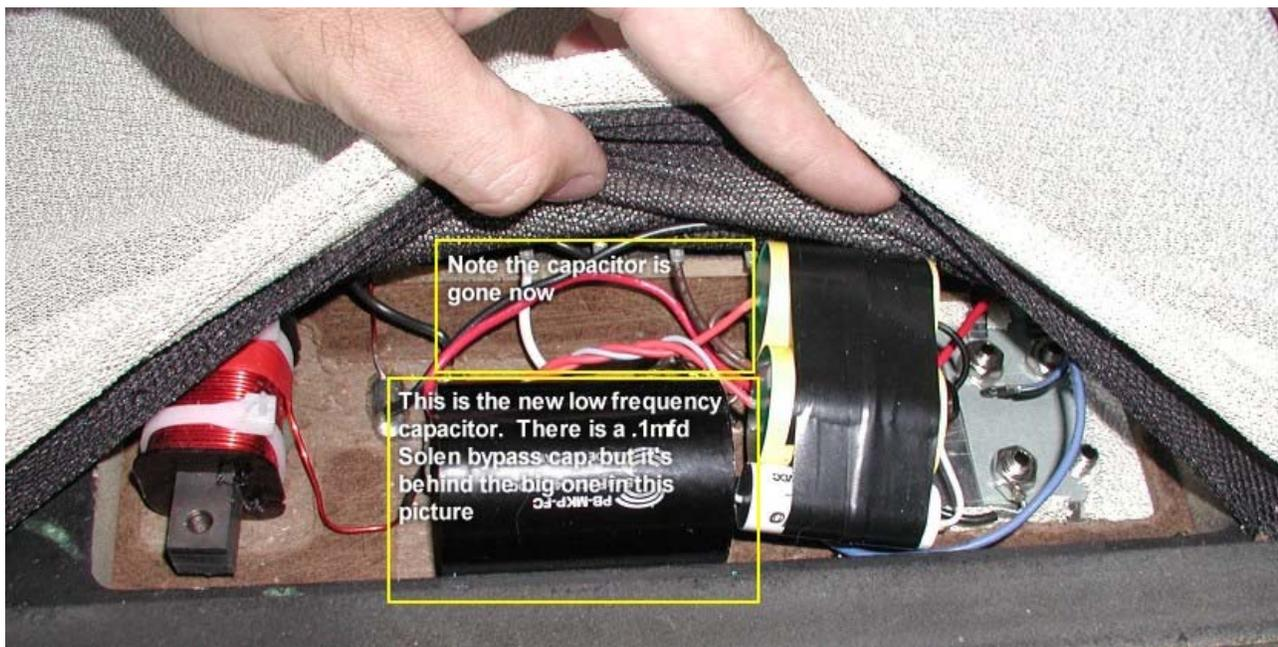
Step 8: Fire it up. It's pretty hard to screw this circuit up since you're just re-soldering to stock locations, and not really changing the circuit, but just in case you might want to verify your work, and possibly hook it up to a cheap amp for the first run just in case, but that's up to you.
