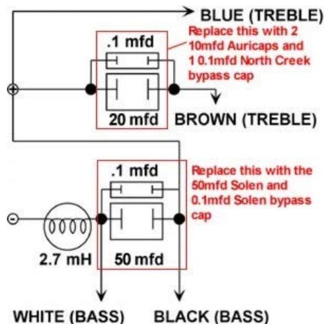
Step 0: If you haven't already TAKE THE FUSE AND JUMPER OUT OF THE CIRCUIT. This makes a noticeable improvement in the clarity of the speaker and requires no soldering. There are a few tweek articles on how to do this. It's completely reversible on the MG12's, unlike other Magnepan's, there is no soldering involved.
