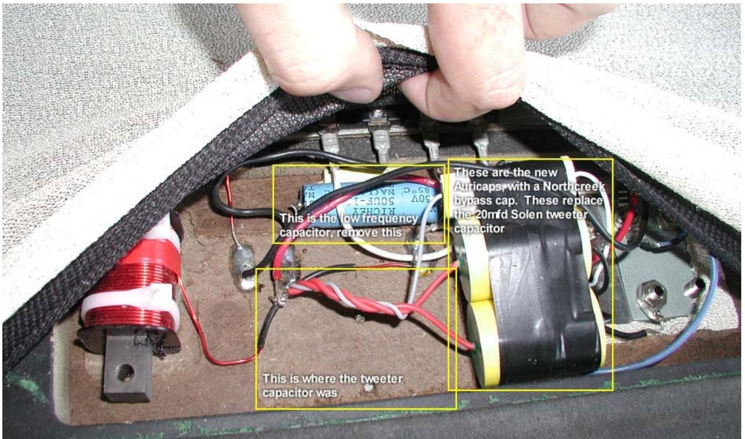
Step 4: Cut the Solen high-pass capacitor out of the circuit. Try to cut as close to the cap as you can, so that you have as much extra lead available, you will be soldering the Auricaps right back where the Solen was, so keep track of things.
